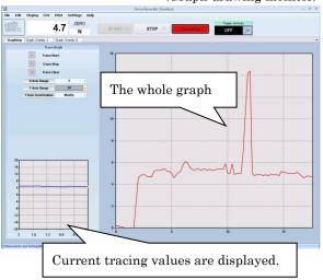
It is possible to start/stop recording automatically when the measured value reaches set points. (Trigger function)\*
