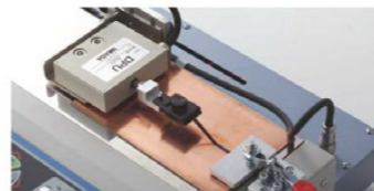
Peel test of copper foil
