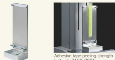
Adhesive tape peeling strength test with P180-200N.
