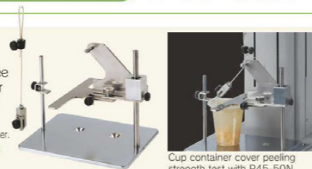
Cup container cover peeling strength test with P45-50N.
