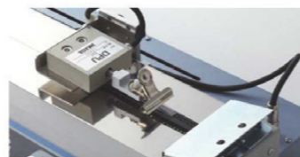
Peel test of embossed carrier tape
