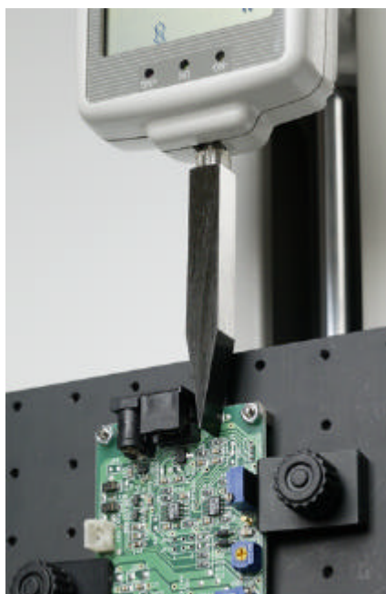
1) TIP 90 degree shear test
