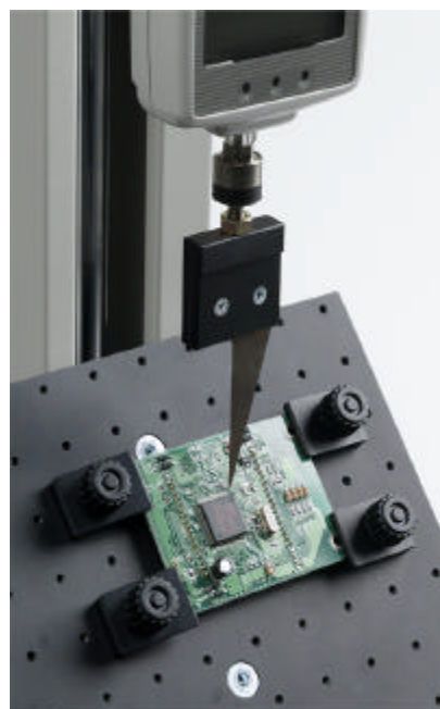
2)QFP 45 degree pull test
