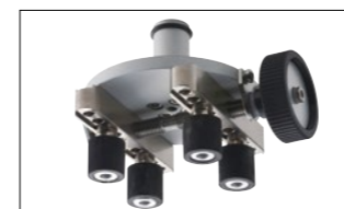
Model: MT-TB Max. torque: 10N-m Sample diameter: φ 20~90mm
