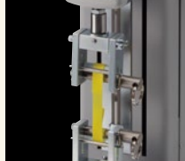
PP band tension strength test with PPC-5000N.
