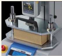
Cardboard box durability test with PR-2500N.
