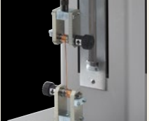
Tensile test of copper wire with WG-1000N
