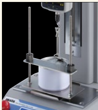
Opening testing for pull-tab of canned food's container.
