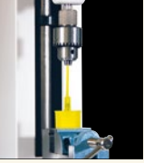
Resin molding tension exception strength test with GC-5.
