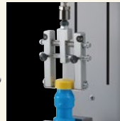
Cap Tension test with SHF-100N
