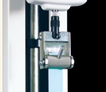
Tape tension strength test with GR-30.
