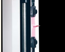
180 degree peel testing of adhesive tapes with FC-21
