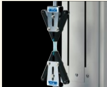
Rubber tension strength test with PGC-0510.
