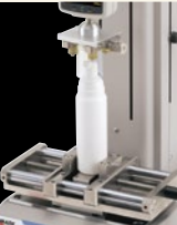
Bottle cap insertion/extraction test with CCJ-100N
