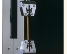
Cable tension strength test with KC-1001.
