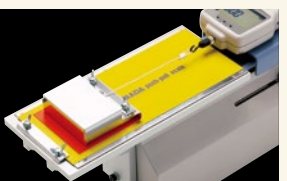
Paper coefficient of friction test with COF2-10N-J
