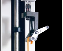
Rubber tape tension strength test with GC-60.
