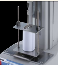
Opening testing for pull-tab of beverage can
