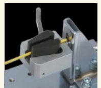
Cable tension strength test with CW-500N.
