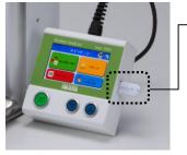
Insert included USB flash drive into the controller.
